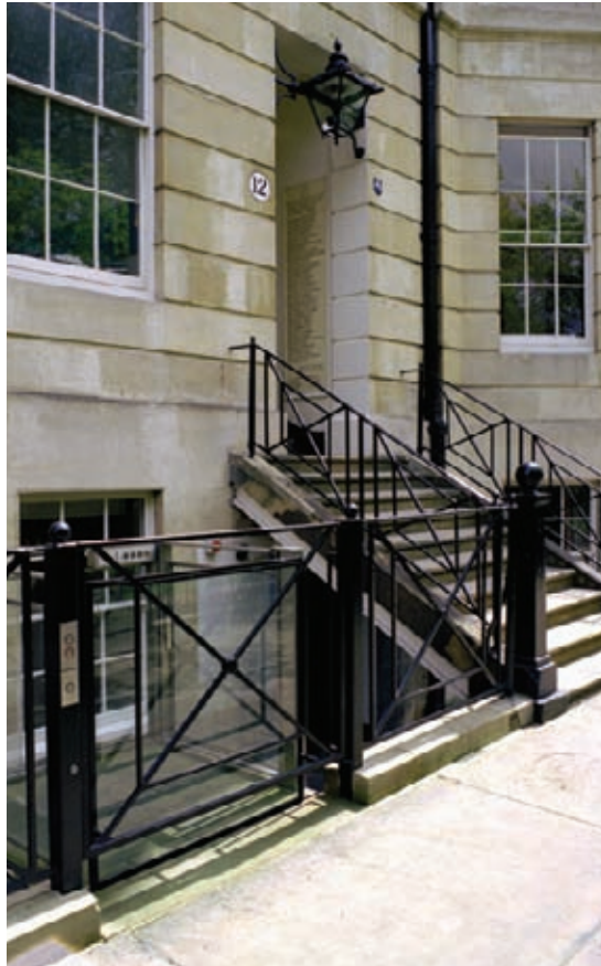
King's Bench Walk, Inner Temple, London. A short-rise platform lift is positioned behind railings where it descends to basement level and connects to the primary circulation routes.
